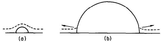
FIG. 5. (a) Bubble surrounded by thermal boundary layer. (b) Bubble growing far beyond thermal boundary layer.
